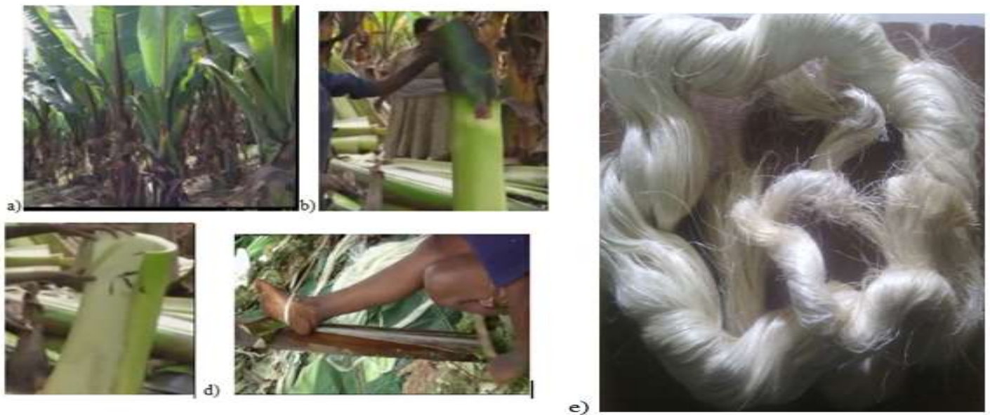
Figure 1. Fiber Extraction from Enset plant; a) Enset plant, b) separating pseudo-stem from leaves, c) slitting thin slice from the inner face of the layer, d) fiber decortication and e) final extracted fiber
