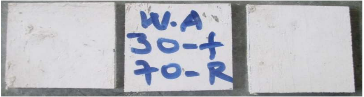
Figure 4. Water absorption specimen
