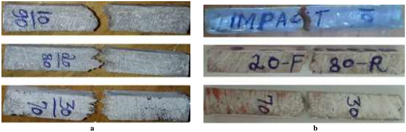
Figure 6. Impact specimens after mechanical failure, a) raw fiber based composite b) alkali treated fiber based composite
