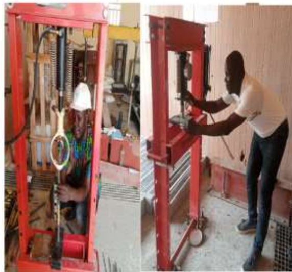
Figure 1 shows a compression Test on steel bar ongoing
