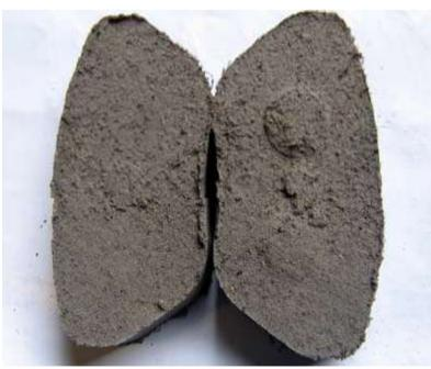
Photo 3.0 (a) Perform of brake pad lining.
