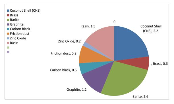
Figure 1: Consistent Ingredient used in the brake pad formulation.
