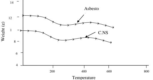
Fig 2: A graph showing comparison of Effect Temperature on Weight of Asbestos of C.N.S. Base Friction Composite.
