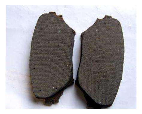
Photo 3.0 (c) Plate of perform and finished CNS-based friction composites.
