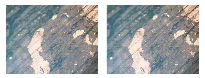
Figure 4.6 SEM Images of Worn out surface
