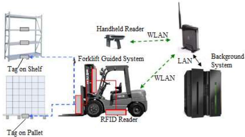
Figure 4. Functionality of RFID based forklift guides system
