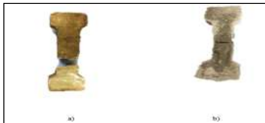
Figure 7. Typical failure occurred in the tensile strength test specimens: a) HSC, and b) HSFRC 0.5 %, 1.0 % and 1.5 %
