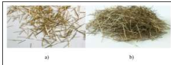
Figure 2. Types of micro-steel fibres: a) 6 mm length, b) 14 mm length
