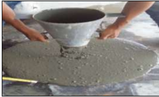
Figure 3. Raise the cone vertically to measure the flowability
