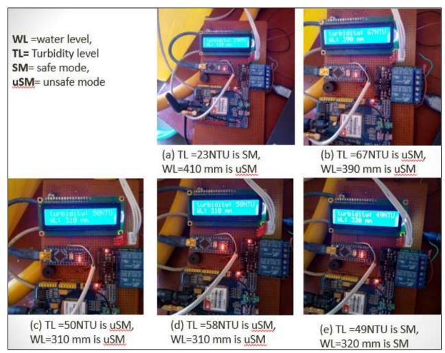
Figure 5: Results from lab system testing
