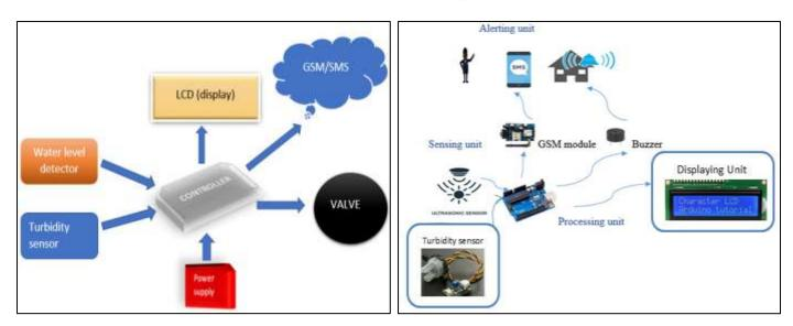
Figure 1.a. Block Diagram
