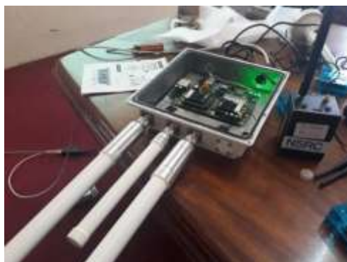
Figure 1: LoRa Gateway and nodes used to deploy our network
