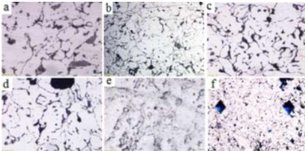
Fig 6. Microstructure images of samples on different percentage of doping Cr. a) 0, b) 0.5, c) 1.0, d) 1.5, e) 2.0%, and f) Vickers hardness indenter trace for 1.5%Cr-doped Fe.
