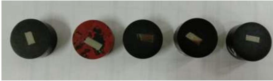
Fig 4. The Metallographic results of samples as a function of Cr content of 0, 0.5, 1, 1.5, and 2% respectively from the left to the right.
