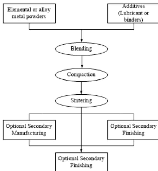
Figure 1. Flow chart of the fundamental powder metallurgy steps.
