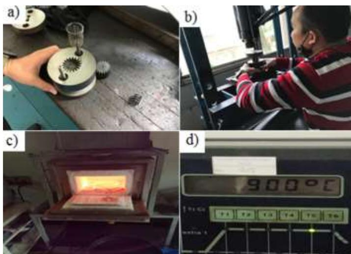
Fig 3. a), b) The mechanical press for the compacting of metal powders and the set of the compaction tooling of the dies, and c), d) Heating furnace for the sintering process.
