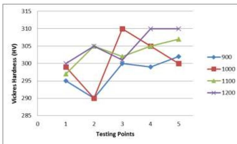
Fig. 10 Behaviour of the hardness of the samples with the variation sintering temperatures on five testing points.
