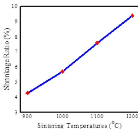
Fig. 8 The shrinkage ratio of the green compact 1.5%Cr-doped Fe sintered at 900-1200<sup>0</sup> C.
