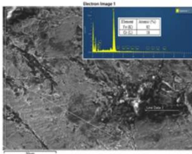
Fig. 5 SEM surface image of 2%Cr-doped Fe sample after the metallographic process.
