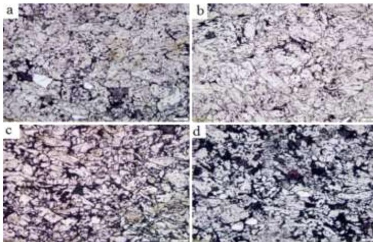
Fig 9. Microstructure images of gears after sintering at a) 900°C, b) 1000°C, c) 1100°C, and d) 1200°C.
