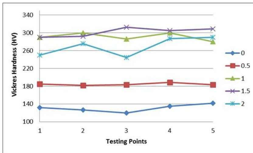
Fig 7. The behavior of the Vickers hardness value of the samples with the different percentages of doping Cr on five testing points.
