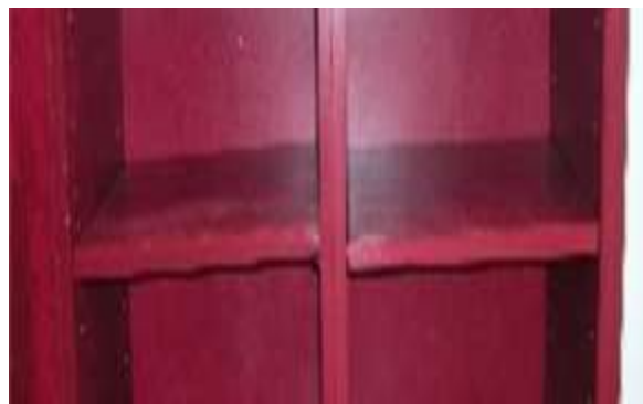
Fig.3. Jute/soy protein composite used as shelving [1]
