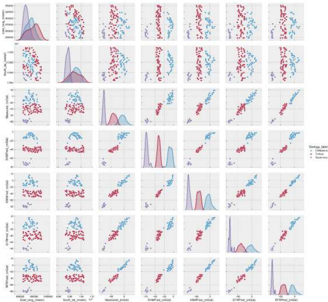
Fig. 7. Compared to measured gravity, all the models showed good result. Random forest has the best performance followed by k-nearest neighbor while Decision tree results are less accurate than those of the two previous models are. In turn, Support vector machine result is not good as that of Decision tree. All the results correlate the regional geology of the study area.
