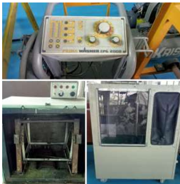
Fig 1. The powder coating equipment consists of Wagner Prima EGP-2008, furnace, and room/box for spray coating.
