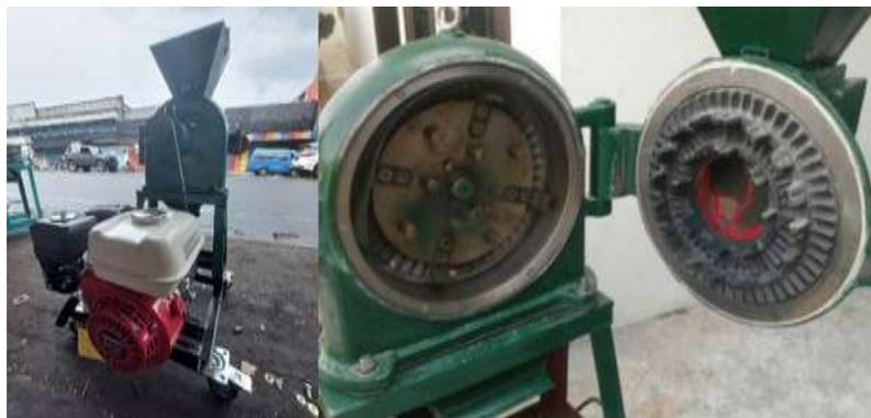
Figure 1. Disk Mill Machine
