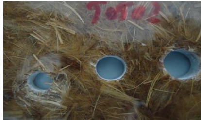
Fig.9.Drilled plate composite material
