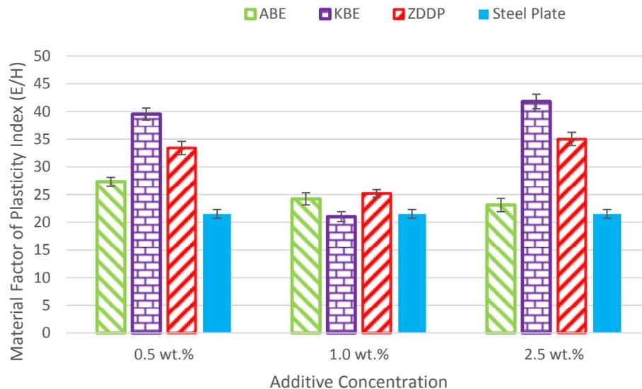
**Figure 7 A comparison of the material factor of plasticity index of wear scar regions for tribofilms formed by different additives at different concentrations**
