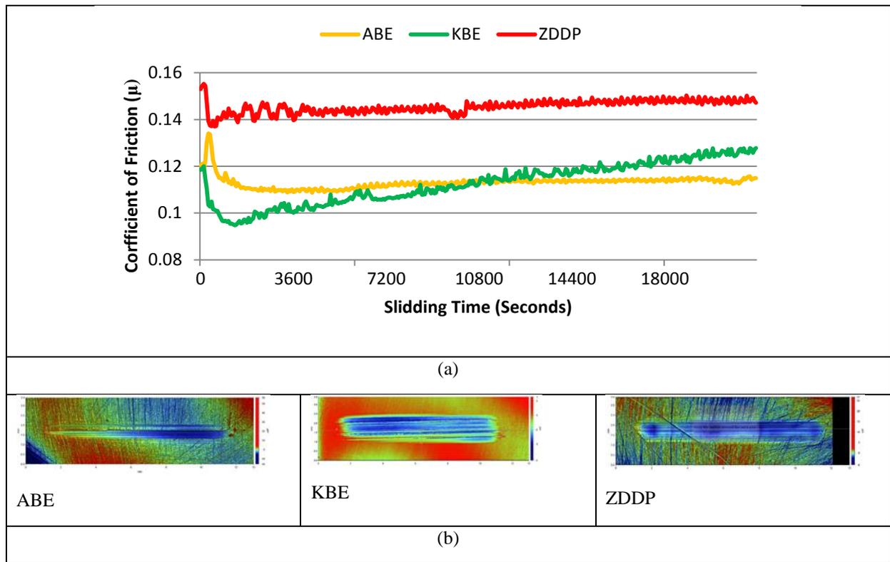
Figure 3 Tribological test results at 0.5wt.% (a) friction behavior and (b) plate wear scars
