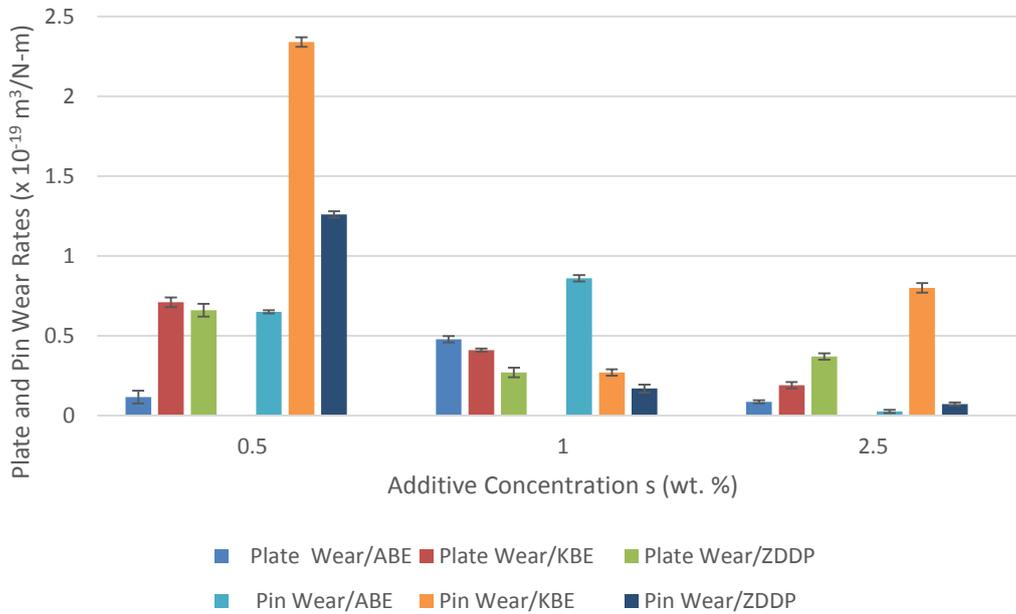
Figure 5 Changes in wear rates of steel samples at different additive concentrations
