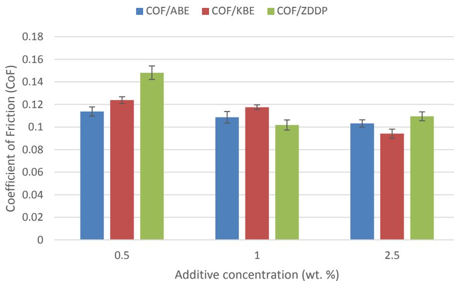
Figure 4: Variation in average coefficient of friction with additive concentration
