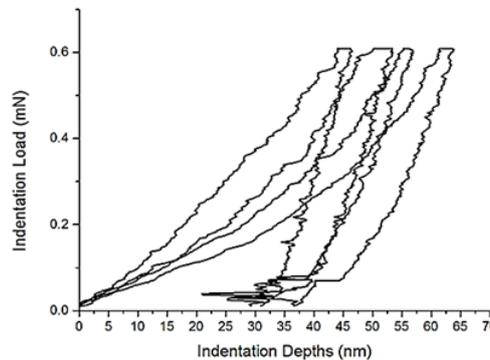
Figure 6 Nano-indentation loading and unloading curves
