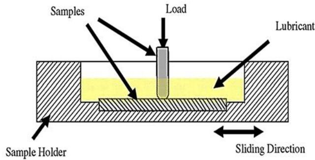
Figure 2 A schematic view of the pin-on-plate reciprocating test rig [21]
