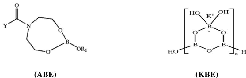
**Figure 1: Molecular structure of the boron additives [18, 19]**
