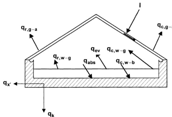
Figure 5: Energy balance of a double basin solar still [12]
