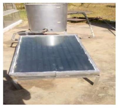
Figure 3: Triple-glazed flat plate collector installed at Sokoto Energy Research Center Sokoto
