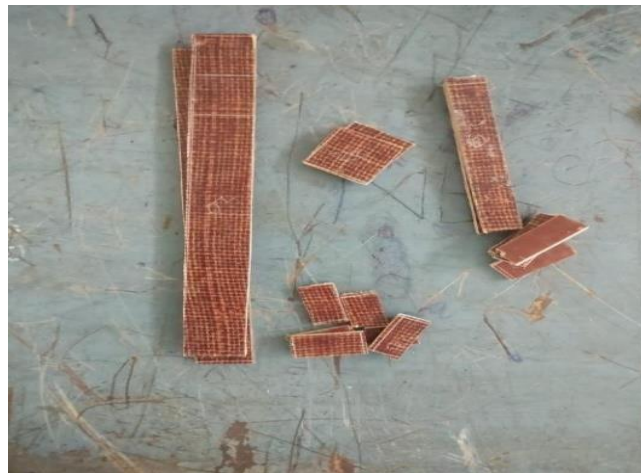
Figure 4.1 Hybridization of bamboo and pineapple fibre with 10gm of agarbatti powder reinforced with Epoxy composite
