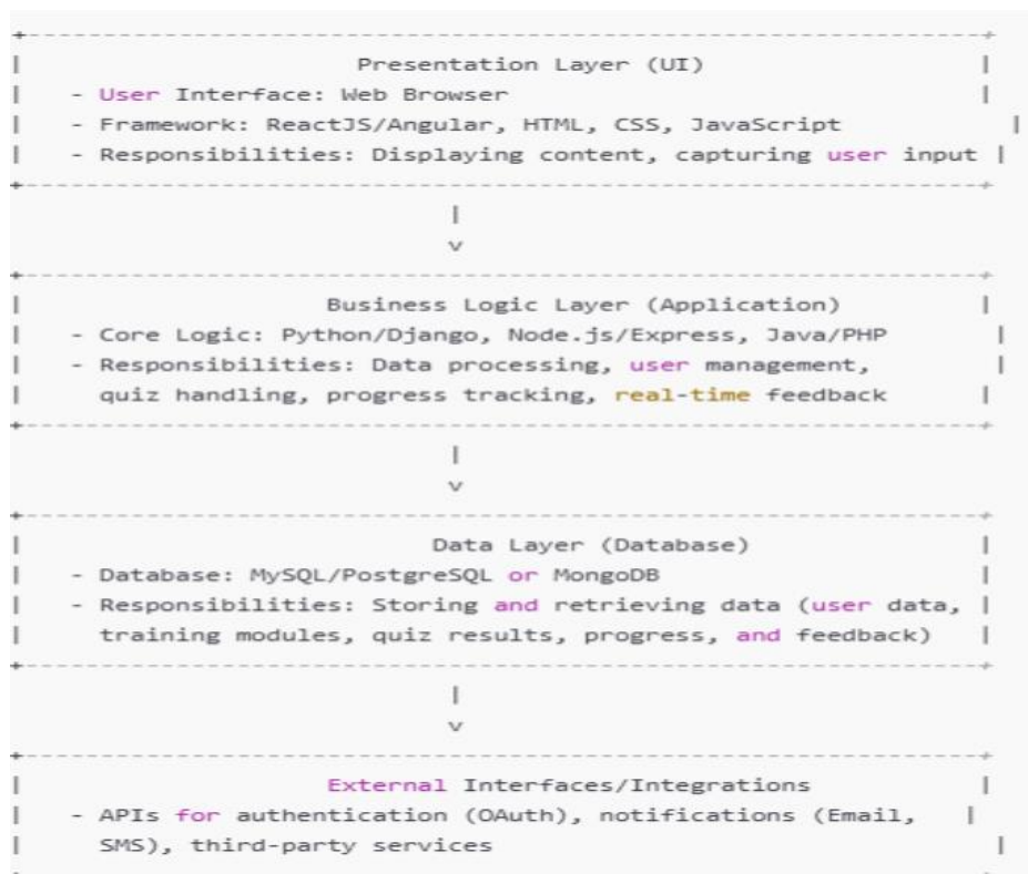
Figure 6: System Software Architecture Design Diagram
