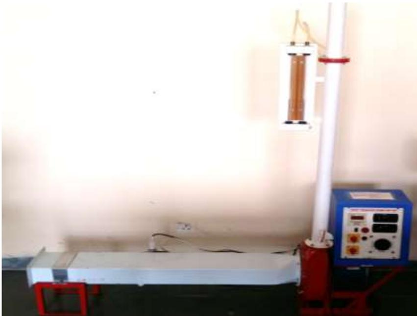
**Figure 1:** Heat transfer experimental setup for a pin fin
