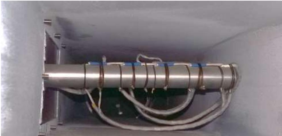
**Figure 2:** The position of the pin fin inside the duct
