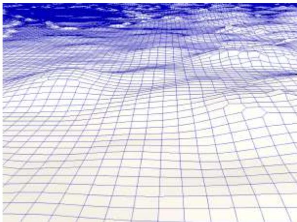
**Figure 8: SnappyHexMesh on Terrain**
