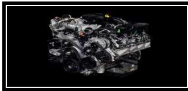
Figure 3: Ford/Peugeot's 2.7-liter V6 uses a cylinder block manufactured out of compacted graphite cast iron [12]
