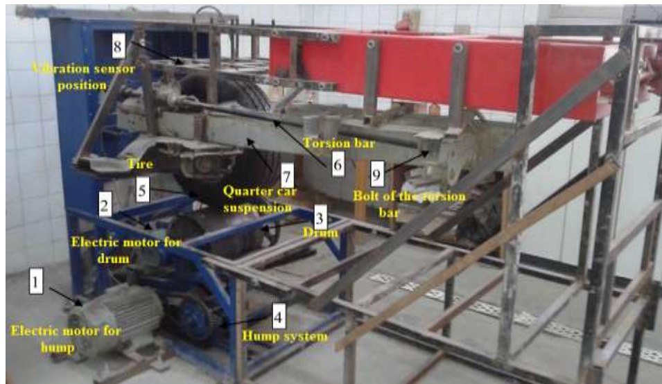
Figure 1. Photo of Torsion bar test rig.
