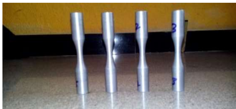
Figure 3: Standard fatigue test specimen after machining
