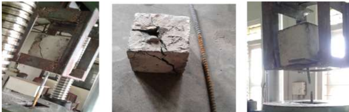
a) Control mix b) Recycled aggregate concrete c) RAC with hybrid fibre
