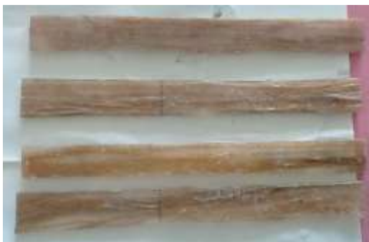
Fig 5. Polyester 96% 4% curaua fiber specimen
