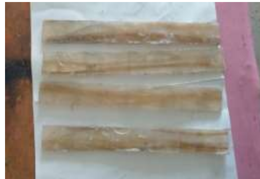
Fig 6. Polyester 94%+3% curaua+3% glass fiber specimen
