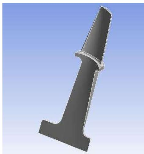
Fig 2. Sector Model of Turbine Blisk
