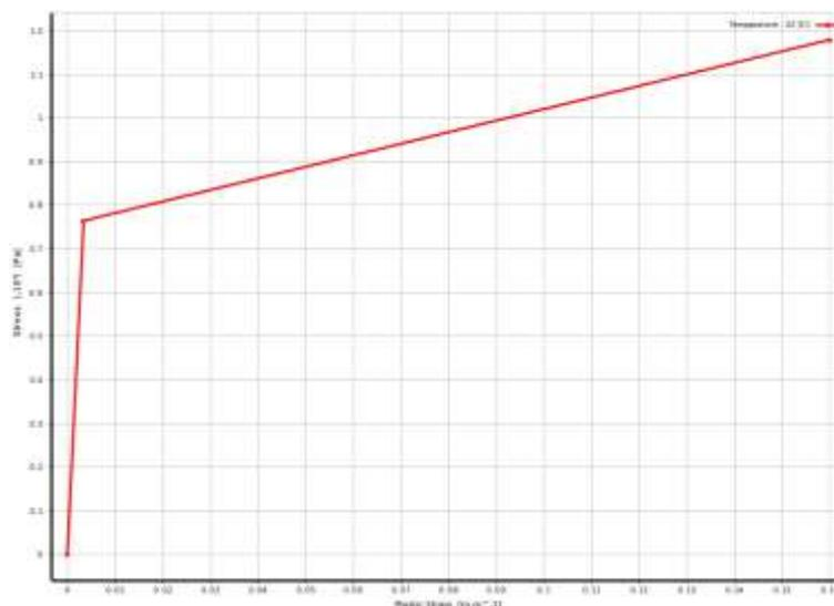
Fig 4. Stress-Strain Curve for Nimonic 105
