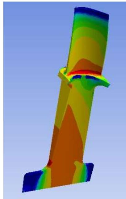
Fig 7. Fatigue Life of Turbine Blisk
