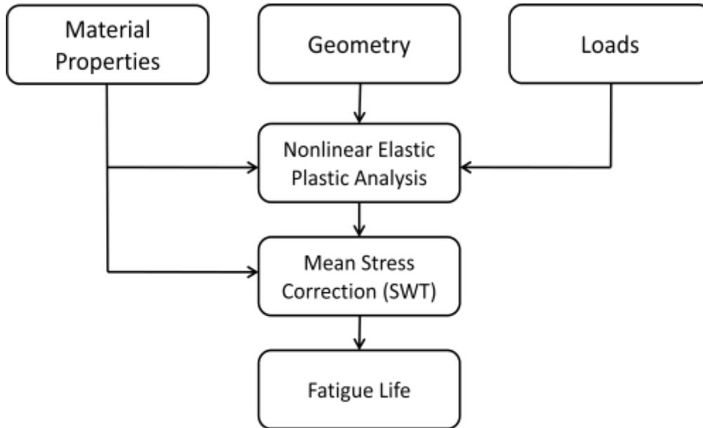
Fig 1. Design Flow Chart of Turbine Blisk
