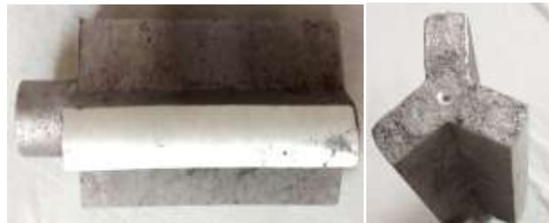
Figure 1: Tri shaped cast composite used for the experiment
