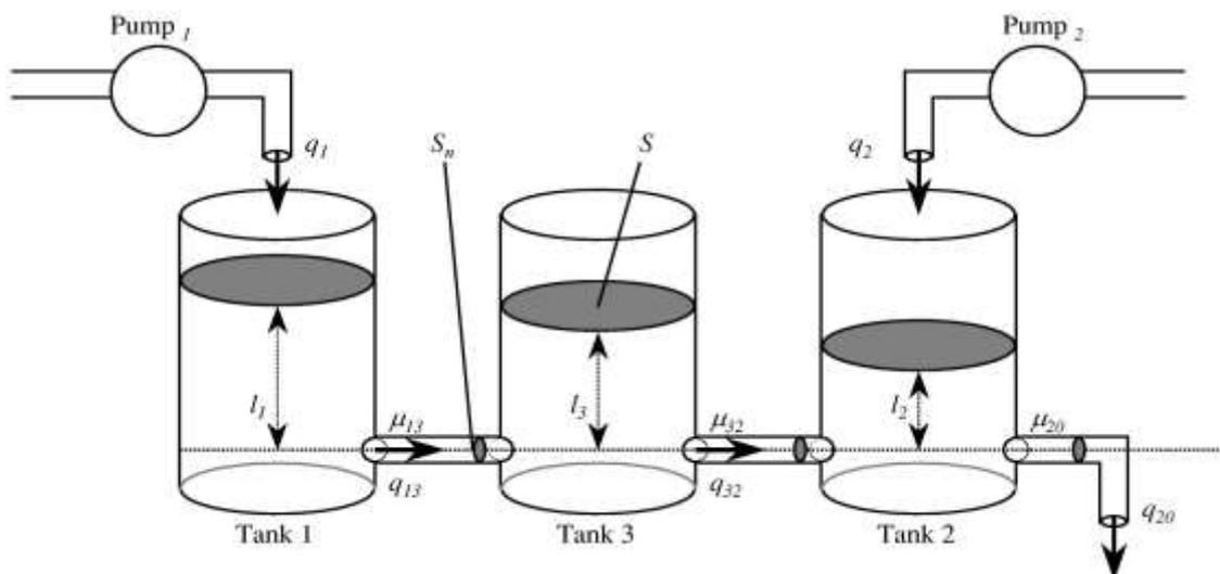
Figure 1: The three tank system schematic (source; Theilliol, *et al.* [11])
