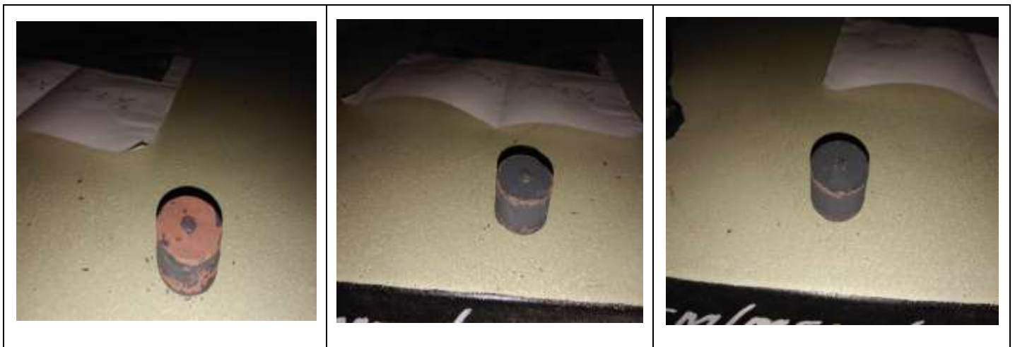
Fig 2.4 Compacted and Sintered specimen
