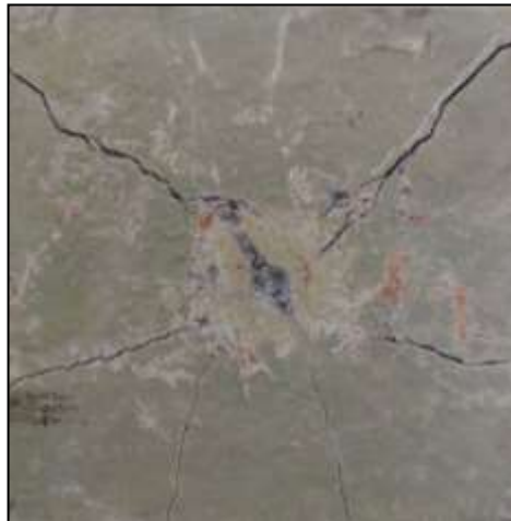
Figure5.4: Slab Specimen during applying of load
