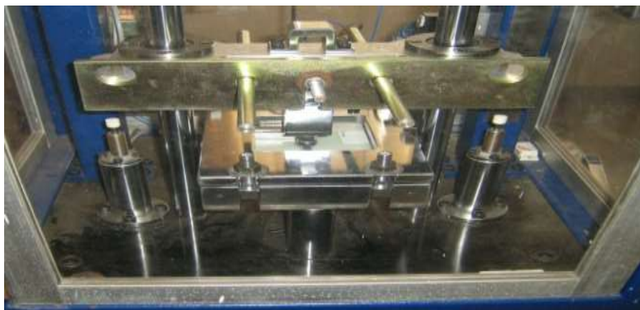
Figure 3. Specimen Clamping Apparatus.
