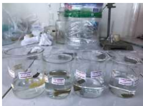
Figure4. Water Absorption Test of Bioplastics for Concentration of (0.5M) HCl
