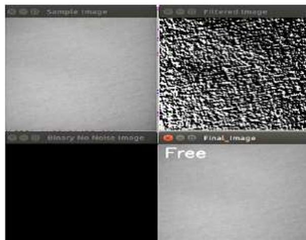
**Fig. 10: Result of No Defect**
