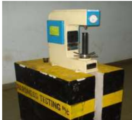
Figure 5 : Rockwell hardness test setup
