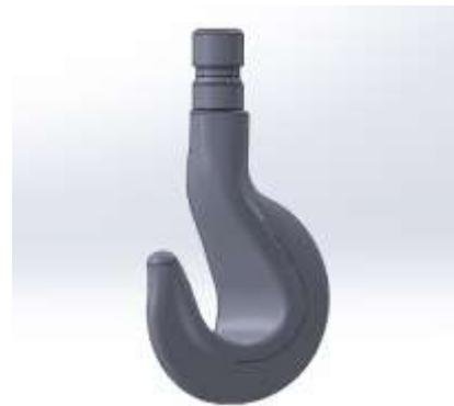
Figure Crane Hook With T-section Cross Section
