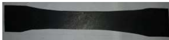
Figure 4: Tensile test specimen
