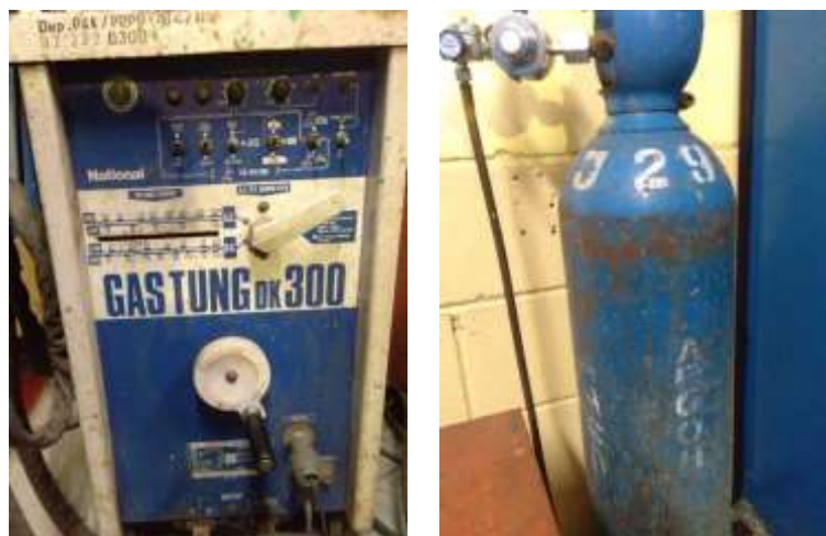
Figure2. GTAW machine and the shielding gas tank
