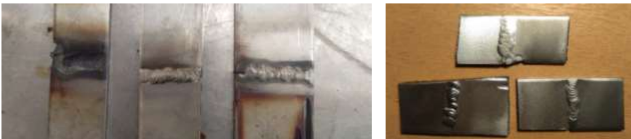
Figure6. Corrosion test piece before and after polishing
