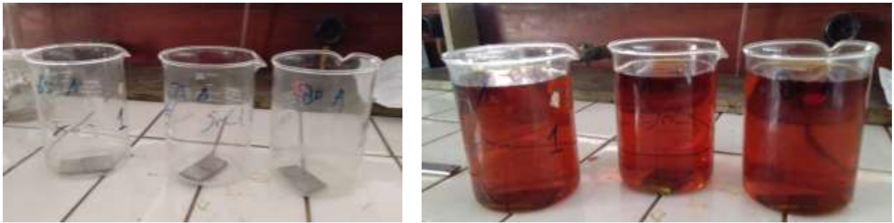
Figure7. Corrosion test piece before and after dipping into the solution.
