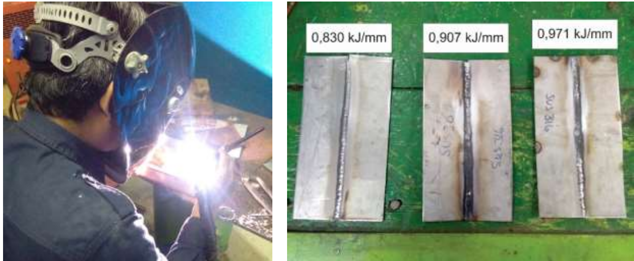
Figure3. Welding process and its results
