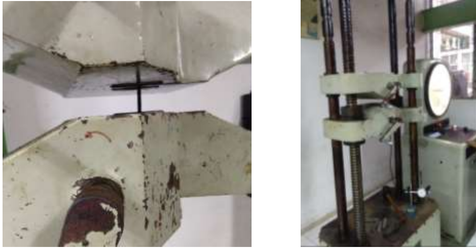
Figure4. Tensile test process in the machine
