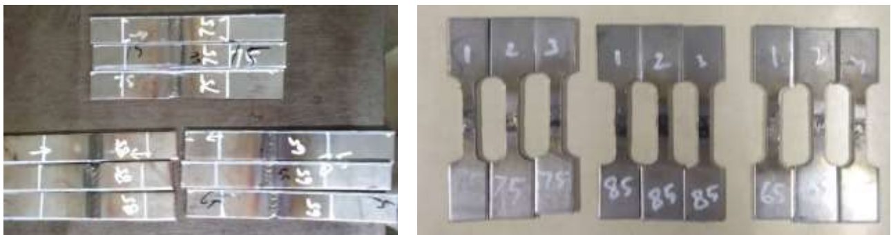
Figure3. Tensile test piece before and after cut according to ASTM E8
