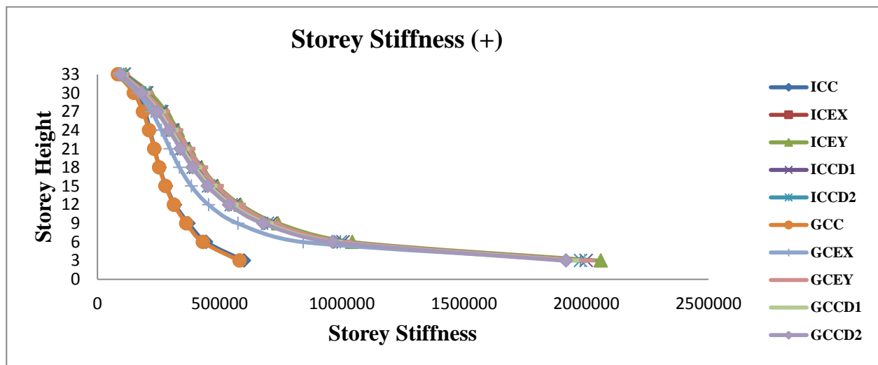
Fig. 17 Storey Stiffness for conventional beam system
