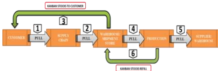
Figure 9: General pull system design for the rubber production company
