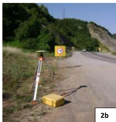
Figure 2a,2b GPS and Levelling Measurements toward Defining Landslide Movements.
