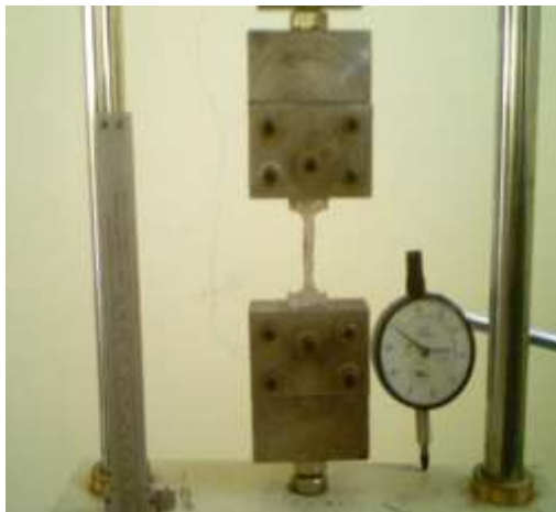
Figure 9-Tensile test specimen setup
