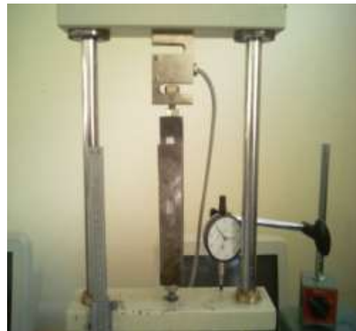
Figure 10-Compressive test specimen setup
