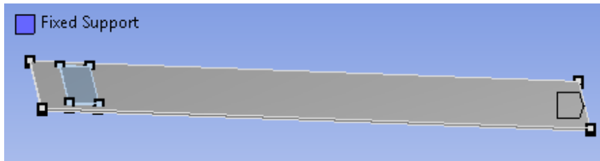
Fig. 7 Finite element model of bimorph beam with support and voltage location
