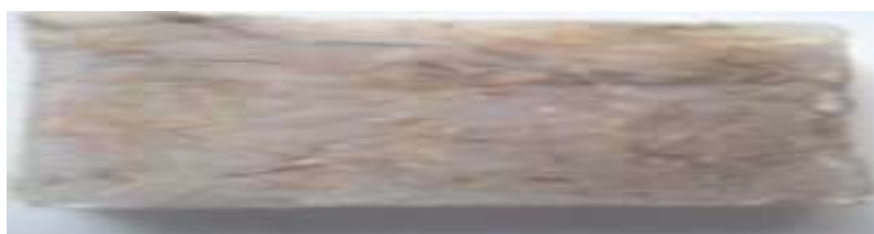
Figure 6:-Sample of palm frond reinforced composite fabricated with injection moulding machine
