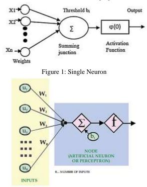
Figure 2: Node (Artificial neuron or perceptron)
