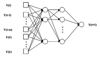
Figure 3: The architecture of the Neural Network
