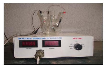
Figure 1. Electrochemical test rig SEP 238C model.
