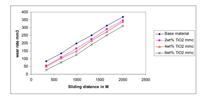
Figure 3. Effect of Sliding distance on wear rate Aluminum alloy & composite material.
