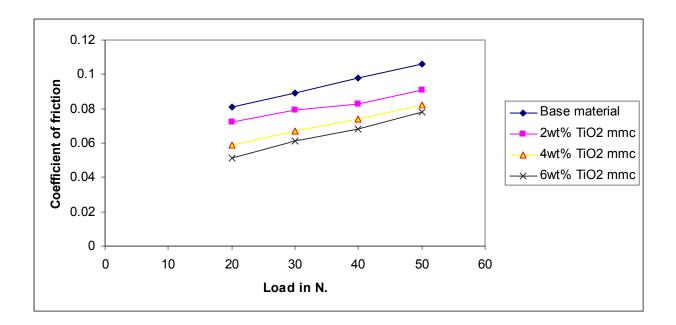
Figure 4. Effect of load on Coefficient of friction on Aluminum alloy & composite material
