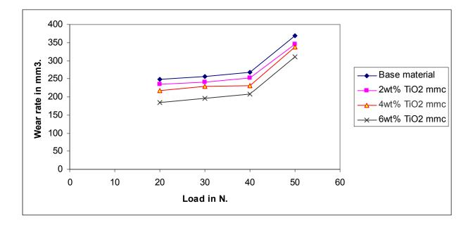
Figure 2. Effect of applied load on wear rate of Aluminum alloy & composite material.
