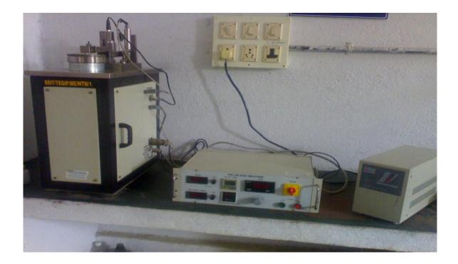
Figure 1. Dry sliding wear test rig.
