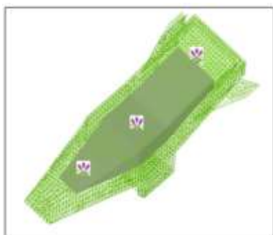
Fig. 3: Hybrid FE-SEA model of the aircraft cabin
