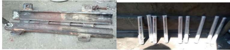
Figure 1.1. Die used for casting Figure 1.2. The Casted specimen
