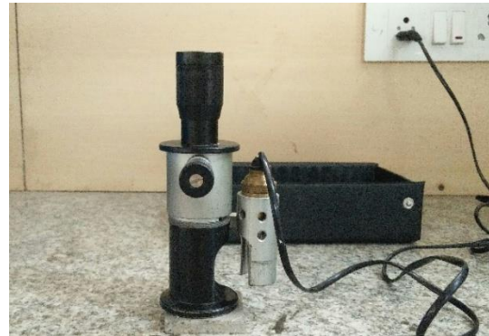
Figure 1.9: Measuring Indentation using Microscope
