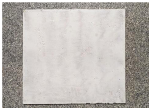
Figure 1. 6: Cured polymer composite panel
