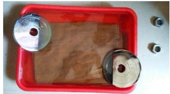
Figure 1.5: Immersion of Jute Mat
