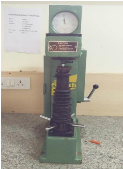
Figure 1.8: Brinell Hardness Testing Machine
