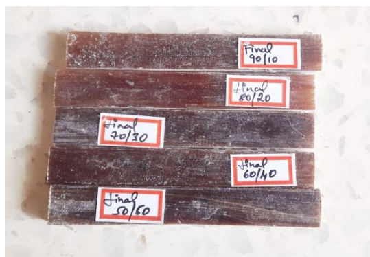
Figure 9: Flexural strength specimens
