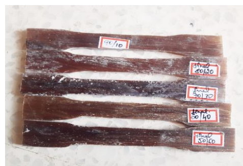
Figure 8: Tensile test specimens
